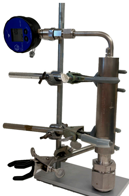
Figure 1. Pressure vessel setup for hydrogen pressure measurements. Customized steel autoclave with pressure gauge designed for hydrogen use.
