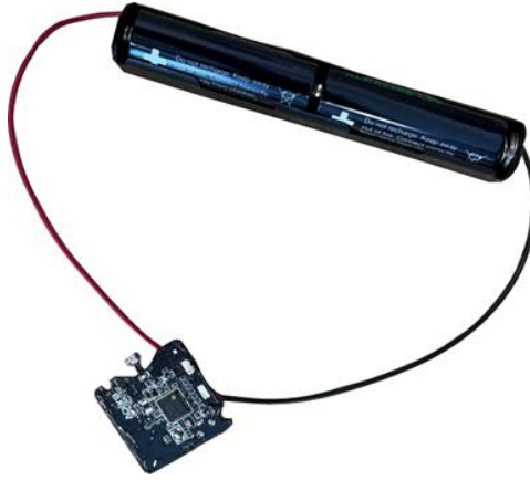
Figure 3: Pressure, humidity and temperature sensor board with attached battery pack [7].
