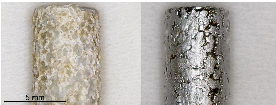
Figure 5: Corroded sample after 1 year exposure time (left) and sample after fully removing concrete residues and oxide (right) [8].
