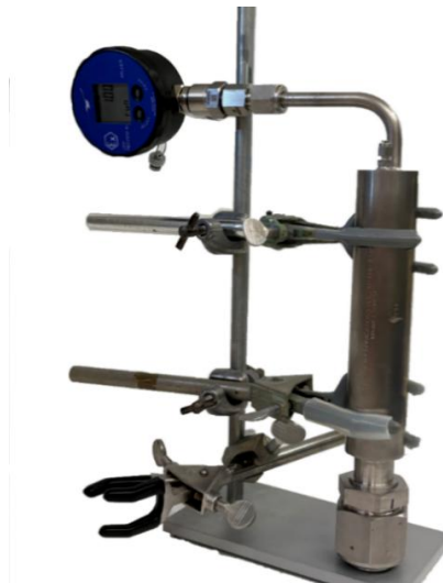
Figure 4: Pressure vessel setup for hydrogen pressure measurements [8].
