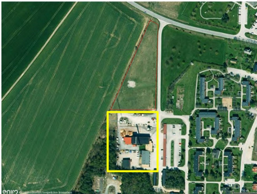
Figure 5: Boiler central – Satellite image of the Hemse boiler plant (Yellow square) and surroundings. The northern area (red triangle) shows available land for installation of solar collectors.
