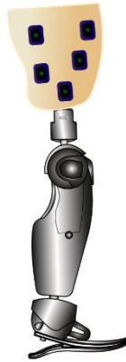
Figure 5 Illustration of five EMG sensors integrated into a custom-made prosthetic socket. The design must accommodate precise sensor placement, which poses challenges due to the movement between residual limb (stump) and socket. These factors can lead to inconsistent signal quality, discomfort for the user, and difficulties in accurately targeting specific muscles.
