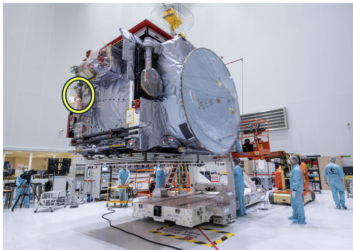
Figure 3.3: JUICE being unpacked after delivery to French Guyana for the launch. SWI can be seen mounted to the left, marked by a circle for extra clarity. Credit: ESA-CNES-Arianespace
