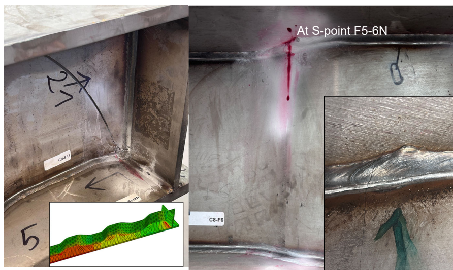
Figure 34 Fatigue cracking at the support in beams C1&C2, and on the compression side in beam C8
