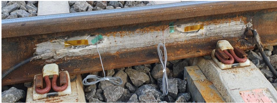
Figure 7.9. Full Wheatstone bridge mounted on the neutral axis of the rail web.
