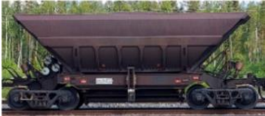
Figure 4.3. (a) Vehicle model with ten DOFs consisting of a car body, two bogie frames and four wheelsets [82], (b) iron ore wagon consisting of a car body and two bogies, each consisting of two wheelsets.
