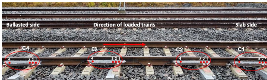
Figure 7.3. An overview of the four clusters (C1 – C4), and strain sensor numbering for each cluster.
