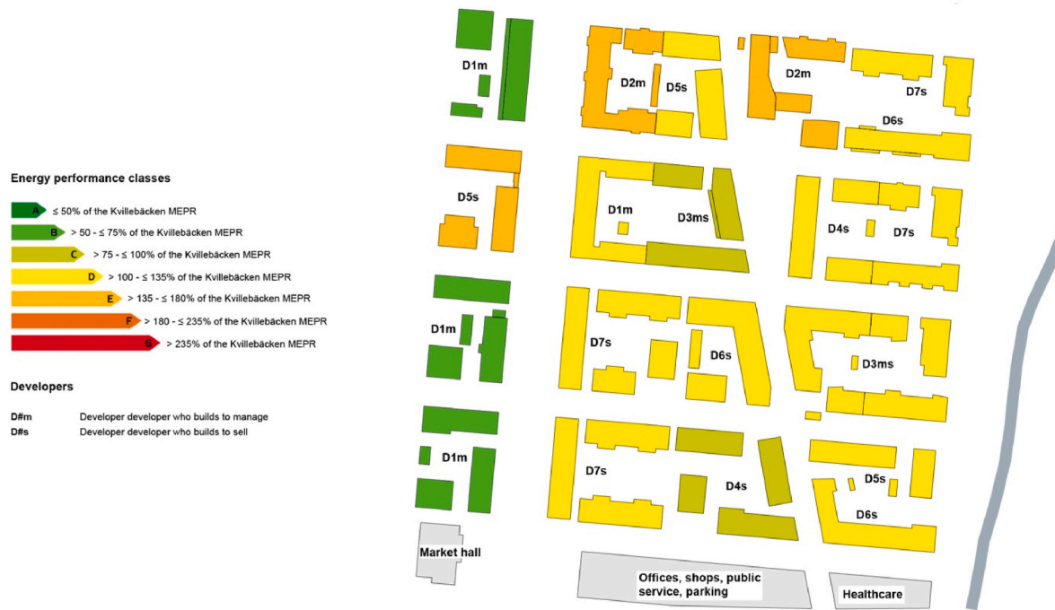
Fig. 3. Energy performance classes of the Kvilebäcken properties. Energy performance data from EPCs have been reinterpreted using specific energy use relative to a reference value of 60 kWh/m 2 per year, corresponding to the stricter MEPR applied in Kvilebäcken. The classes were defined as percentage bands around this reference value (see Table 1) to ensure consistency in the comparison of EPCs issued between 2015 and 2020.
