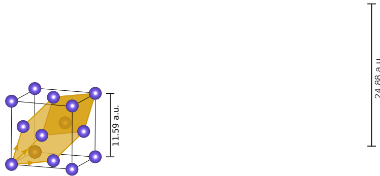
Figure 1: Left: The face-centered-cubic crystal structure of solid xenon, with the primitive rhombohedral unit cell shaded in gold. The arrows indicate the primitive lattice vectors. The experimentally measured value of the cubic lattice parameter extrapolated to 0 K is 11.59 a.u. [33]. Right: Representative supercell of liquid xenon extracted from our Monte Carlo simulation (see details in Sec. 3.4) and used as input for liquid-phase DFT calculations. This region was randomly sampled from the generated atomic distribution and contains 30 atoms within a cubic cell with a lattice parameter of 24.88 a.u., yielding the measured atomic density inside the detector \rho_{det} = 1.949 \times 10^{-3} atoms/a.u. 3 [34, 35].
