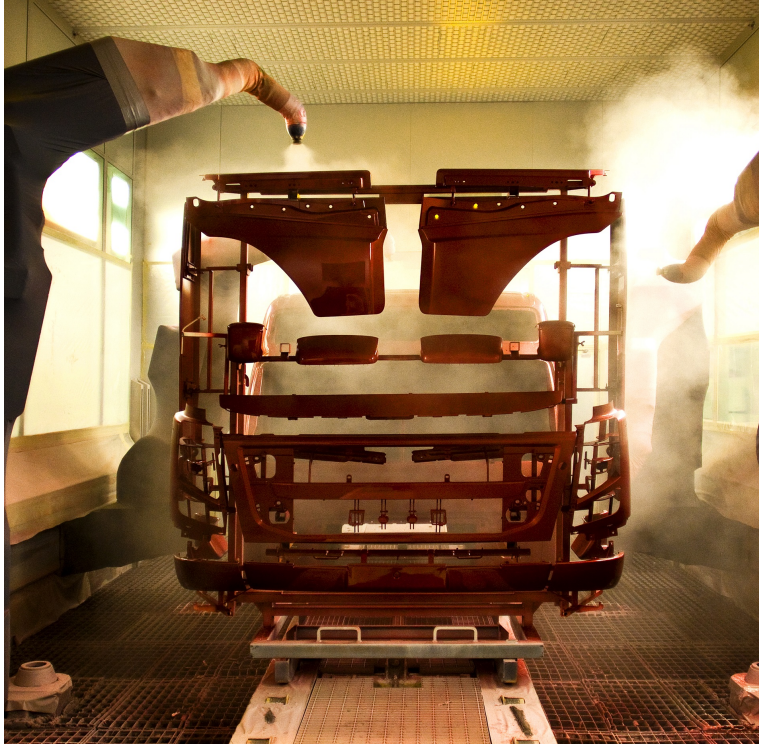
Figure 5.1: An example of an automated painting booth, where robots are painting parts of a Volvo truck suspended on a rack. Image courtesy of AB Volvo.
