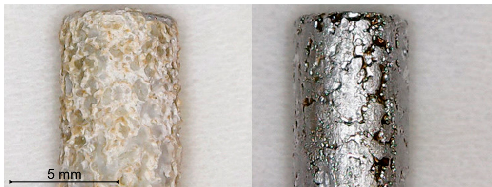
Figure 2. Retrieved R2 alloy sample after one year of exposure embedded in concrete (left) and sample after fully removing concrete residues and oxide (right).
