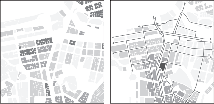
FIGURE 6.4 Density measured as an area metric (left) and as a location metric (right), more precisely as population per urban block (left) and accessible population within a radius of 1,000 meters following the street network from each parcel (right). The same population data is used in both examples. (Darker shading means accessibility to larger populations.)
