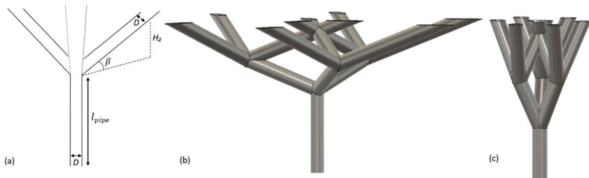
Fig. 1. (a) Schematic depicting the definition of angle of branches \beta . 3D models with the narrowest and widest trifurcation angles investigated for three-level designs with trifurcation angles of (b) 20° and (c) 65°. The total height was divided into three levels: the bottom level has 1 pipe, the middle level has 3 pipes, while the top level has 9 pipes. The inner diameter of each pipe ( D ) is 48.6 mm.
