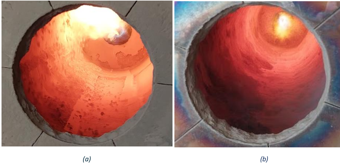
Figure 5 (a) Inner surface of the kiln operated with crushed limestone, where the lifters along the refractory wall are clearly visible and no coating layer is formed. (b) Inner surface of the kiln operated with fine raw meal, where the lifters are obscured by the buildup, indicating the formation of a continuous coating layer.
