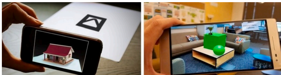
Fig. 9. Example of marker-based AR to aid positioning of virtual objects.
