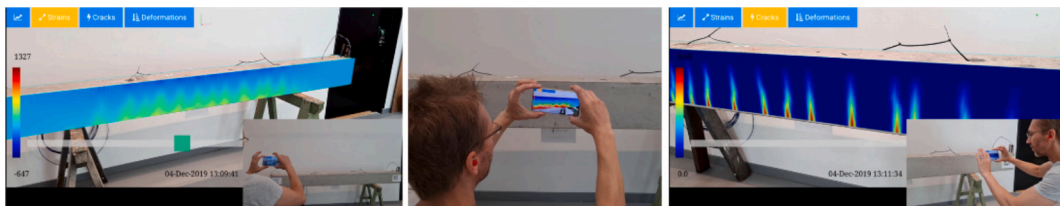
Fig. 15. Data visualization on the beam through the AR environment after alignment.
