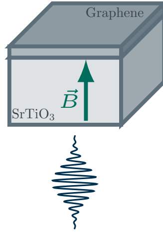
Figure 4.2: The experimental setup consisting of a sample of SrTiO 3 and a layer of graphene placed on top of it. A circularly polarized laser pulse is applied to the SrTiO 3 sample. Thus, a magnetic field \vec{B} is expected to emerge due to the axial phonons driven by the laser pulse.
