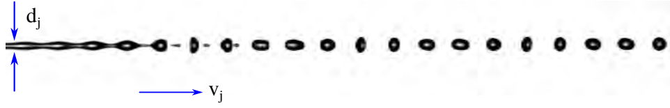
Figure 1.2: A laminar liquid jet, issued from an orifice with a diameter of d_o = 100 \mu\text{m} , is subjected to regular, controlled perturbations at a frequency of f_d = 12.0 \text{ kHz} (Lokesh, 2017).
