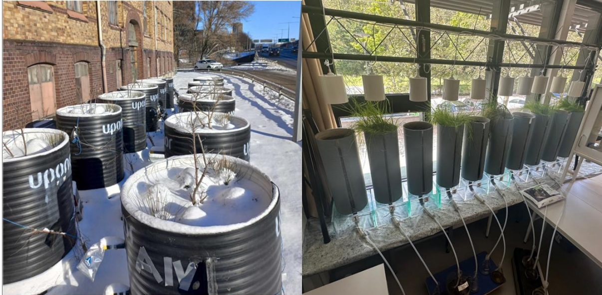
Figure 4. Investigations of the retention and transport of TWP through different soil types were conducted at two scales: at a larger scale in a rain garden pilot facility (Paper V) at Gårda with bioretention filters with different sorption materials, and in a controlled laboratory setting using ten soil-filled columns with and without biochar and grass in the top layer (Paper IV).
