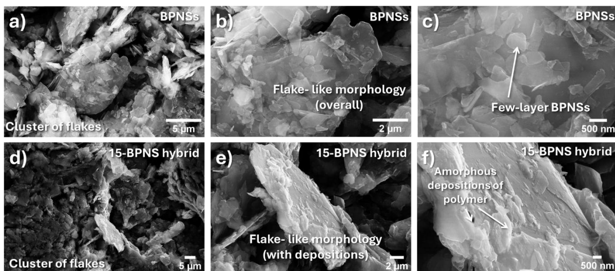
Figure X4. SEM images of (a-c) BPNSs and (d-f) the 15-BPNS hybrid. Flake-like morphology is present in both cases; in contrast, amorphous polymeric depositions can be observed for the 15-BPNS hybrid (e,f).
