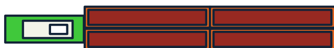
Fig. 5. A typical inland navigation convoy is made of one pusher and four barges.
