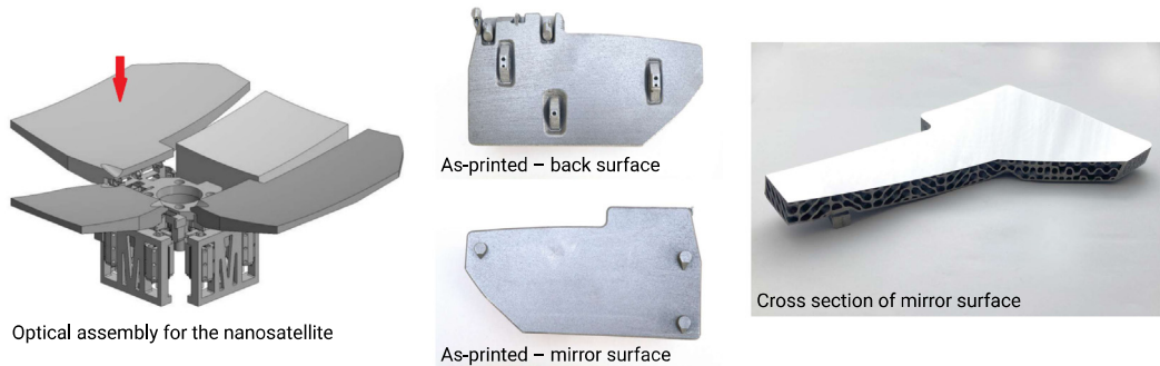
Fig. 45. (left) the nanosatellite optical assembly highlighting the mirror petal; (middle) the as-printed design that underwent XCT acquisition; and (right) a cross section through the reflective surface showing the internal lattice.
