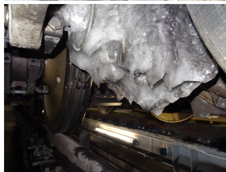
Figure 2: Derailment on the Iron Ore line 2023. Embankment collapse 1918. Under-carriage and brake on Iron Ore loco covered with ice.
