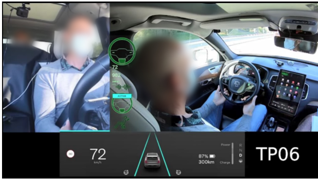
Figure 4: Example screenshot from the video data used to extract the observation data. Shows a participant holding the steering wheel while driving with the Level 3 DAS active.
