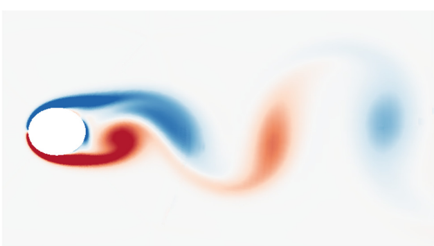
FIG. 11. Vorticity for flow past a cylinder at Re = 200 .
