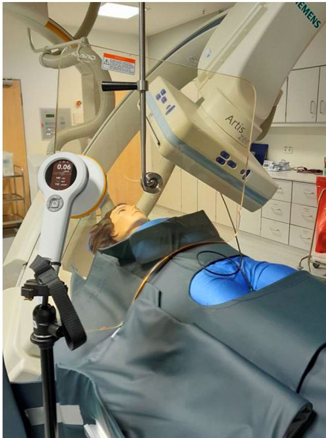
Fig. 2 The configuration of the ERPD set-up for intervention using femoral access, having the Raysafe 452 dosimeter at a height of 160 cm
