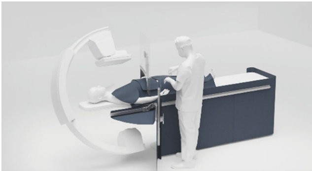
Fig. 1 The ERPD, MasterPeace (Texray AB, Sweden), displaying the foldable over-table shields designed to reduce scatter radiation emitted from the patient; and the table-side shielding components allowing unimpeded C-arm angulations while reducing scatter radiation below the table
