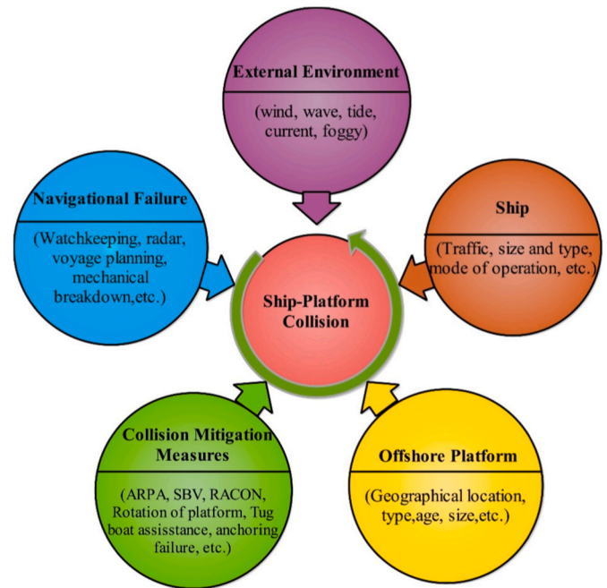
Fig. 8. Key elements in collisions between ships and offshore structures [95].
