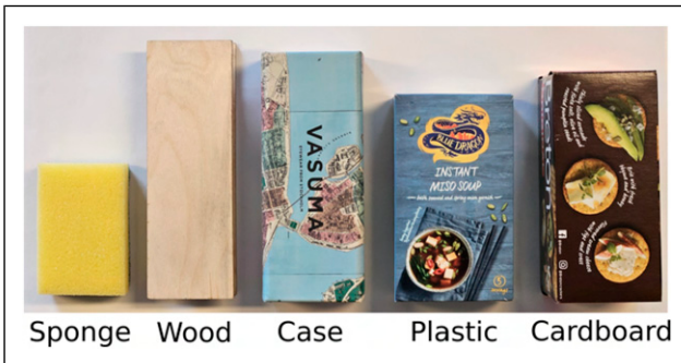
Figure 17. Test objects, the sponge is highly deformable, the wood object has a plywood surface and is rigid. The spectacle case has a synthetic leather material. The plastic object is a plastic covered cardboard box. The cardboard box has a paper finish.
