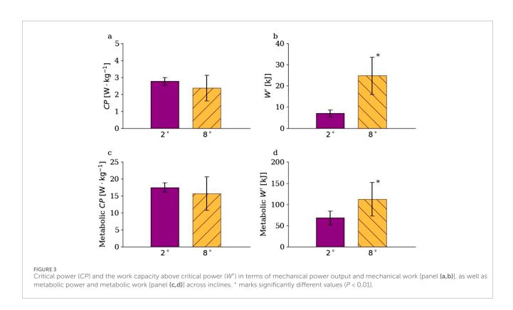
on a motorized treadmill. Its main findings were that: 1) W' and  $P_{an}$  showed a substantial increase with a steeper incline, whereas 2) CP demonstrated a moderate decrease at an 8° incline, although this decrease was not statistically significant. Accounting for the estimated effect of changes in GE across predictive trial conditions lowered the difference in W' between inclines, but it remained statistically significant.
