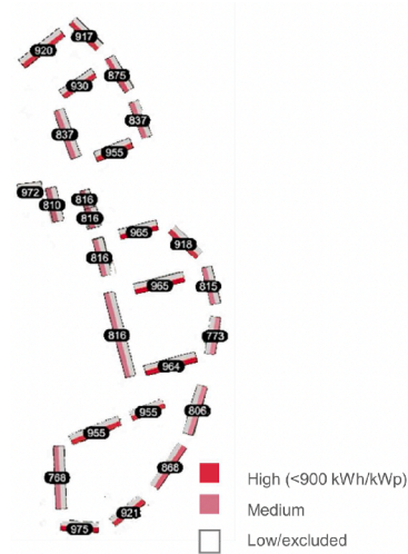
(b) Nominal PV yield (in kWh/kWp a year) per roof segment, calculated using PVGIS under standard configuration assumptions. The roof segments are classified into high (>900), medium- (750–900), and low-performing (<750), guiding the selection for feasible PV deployment in the MILP optimization model.
