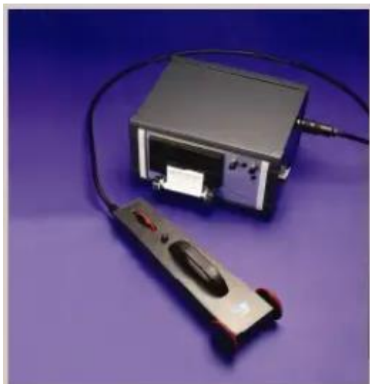
Figure 4.2: Hull roughness Analyzer used to measure roughness of hull surface
