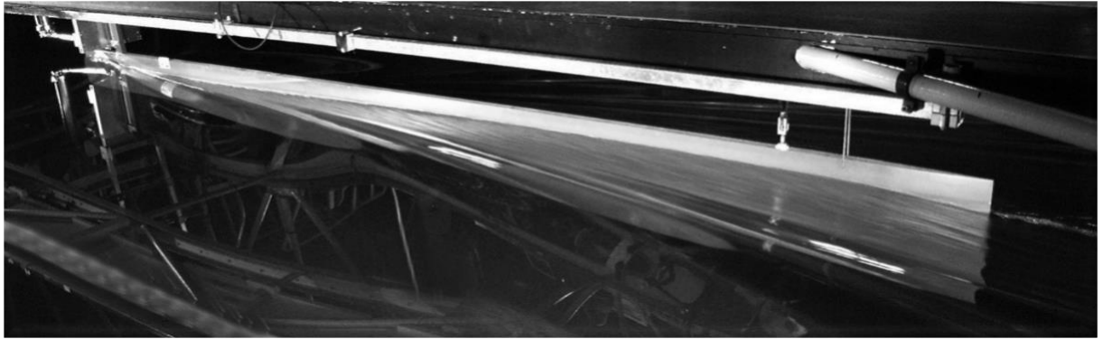
Figure 5.1: Flat plate in towing tank at SSPA Maritime center
