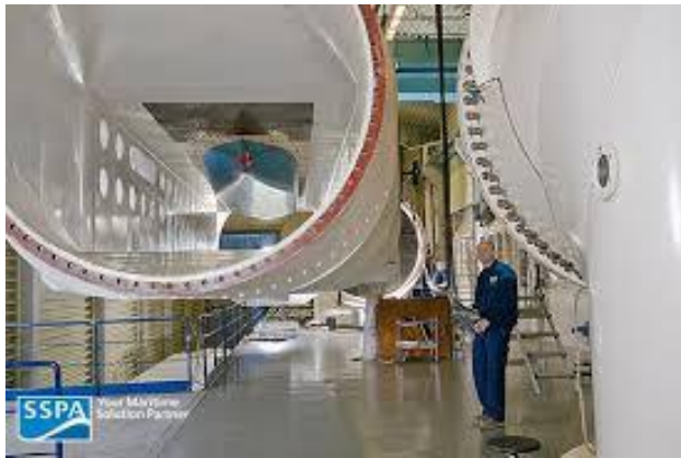
Figure 5.2: Cavitation tunnel at SSPA Maritime Center
