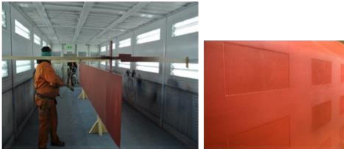
Figure 4.4: Simulated aged and damaged coating
