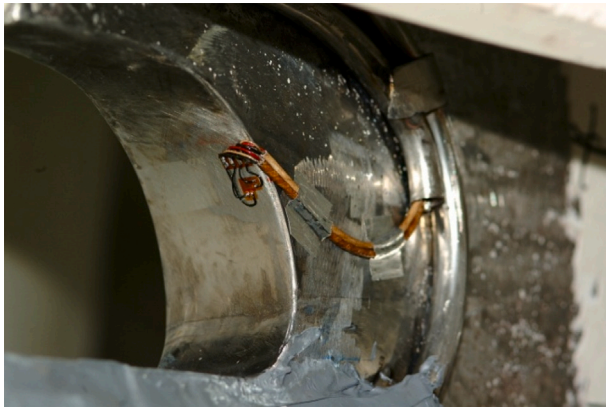
Fig. 7. Strain gauge mounted at the transition from the crown to the runner blade on a Francis turbine. Reprinted with permission from Gagnon et al. [12].
