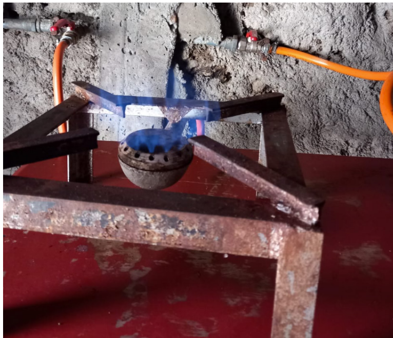
Figure 11. Locally fabricated and distributed biogas stove
