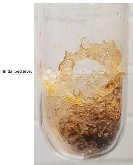
Fig. 4. Solid residue (21 %) left inside the reactor after the experiment was stopped at the end of Stage 1. The liquid yield from this test was 77 %. Most of the polymer at the reactor's centre had decomposed, leaving a layer of mostly un-depolymerised material on and near the reactor wall.
