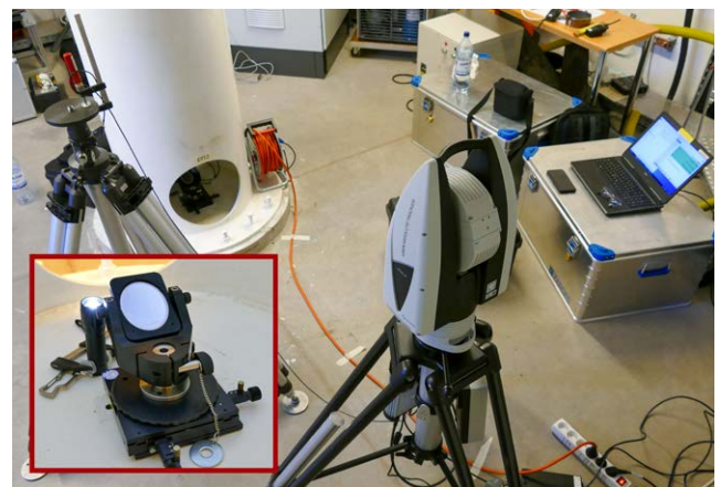
Fig. 2: Laser tracker AT960 in front of the side opening of the tube. An SMR is observed via a plane mirror located centrally inside the tube. The plane mirror is mounted on a cross slide and shown in detail.
