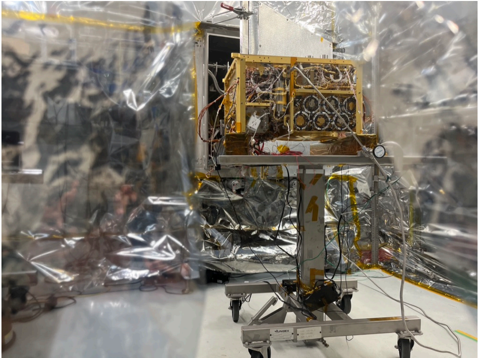
Figure 4. The copy of Sample Analysis on Mars (SAM) instrument at NASA Goddard Space Flight Center. The instrument is behind a so called “clean tent” that protects it from contamination. Photo from fieldwork.
