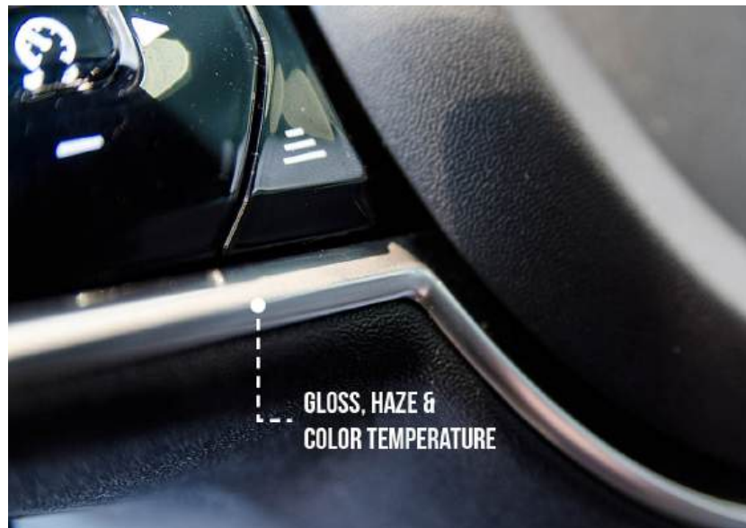
Figure 47. A picture illustrating the chrome-plated plastic component in the interior design for the topical research project from Paper IV. Gloss, haze, and color temperature were the sub-design elements that were in focus for the surface evaluation (Bergman et al., 2016).
