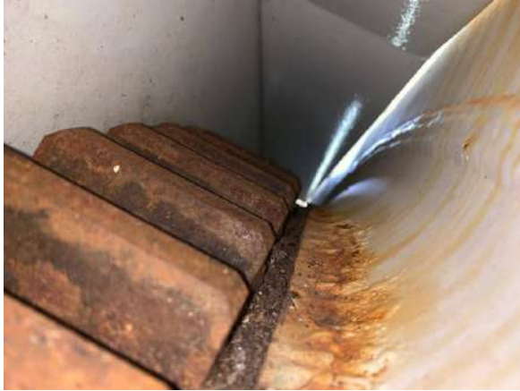
Fig. 4 Rust in RAEGE Santa Maria radiotelescope pinions.
