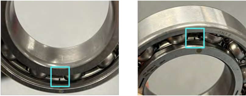
Figure 2.4: The test ball bearings with single ORF (left) and single IRF (right).
