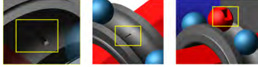
Figure 3. (left) Fault on the outer ring; (middle) fault on the inner ring and (right) fault on the ball.
