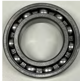
Fig. 1: The experimental setup of the test rig: (a) the arrangement of the sensors and the components (b) the location of the accelerometer (c) the standard SKF 6007-2Z deep-groove ball bearing.
