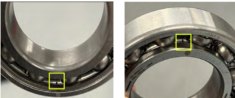
Fig. 2: The artificial ORF (left) and IRF (right) are created by laser machining.
