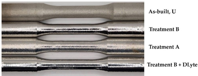
Fig. 5 Qualitative observation of the fatigue samples in the top view illustrating the observable difference in surface quality
