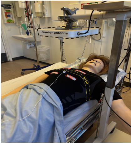
FIGURE 2. Experimental setup for the four-tag placement scenario. The breathing pattern is measured by both the RFID system and a PZT belt. The reader antenna, tags, and PZT belt were highlighted with black, red, and yellow dashed outlines, respectively.
