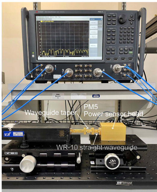
FIGURE 4. Measurement set-up. Photograph showing the reflection coefficient measurements of the PM5 power meter and a waveguide taper.
