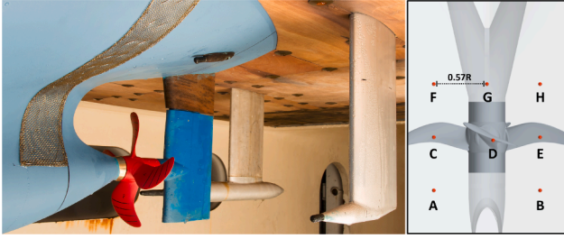
Fig. 2. Ship mounting in the cavitation tunnel (left) and top view for the pressure transducers placement during the model tests.
