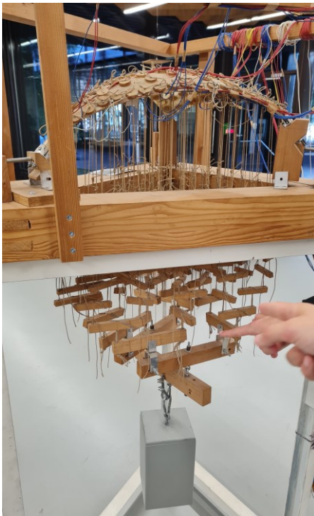
Figure 1: Model by Heinz Isler at an exhibition organized by Giulia Boller of a shell structure loaded by a whippletree
