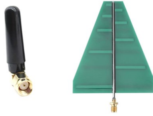
Figure 1.3: An example of a monopole antenna (on the left) and a directional antenna (on the right).
