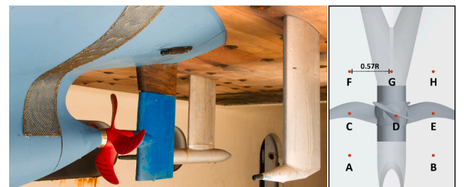
Fig. 2. Ship mounting in RISE cavitation tunnel (left) and top view for the pressure transducers placement during the model tests.
