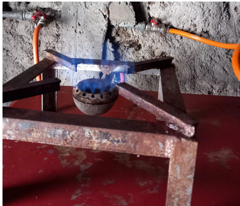
Figure 11. Locally fabricated and distributed biogas stove
