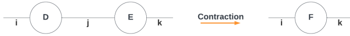
Fig. 5. The tensors D and E are contracted into a single tensor F, with indices i and k.
