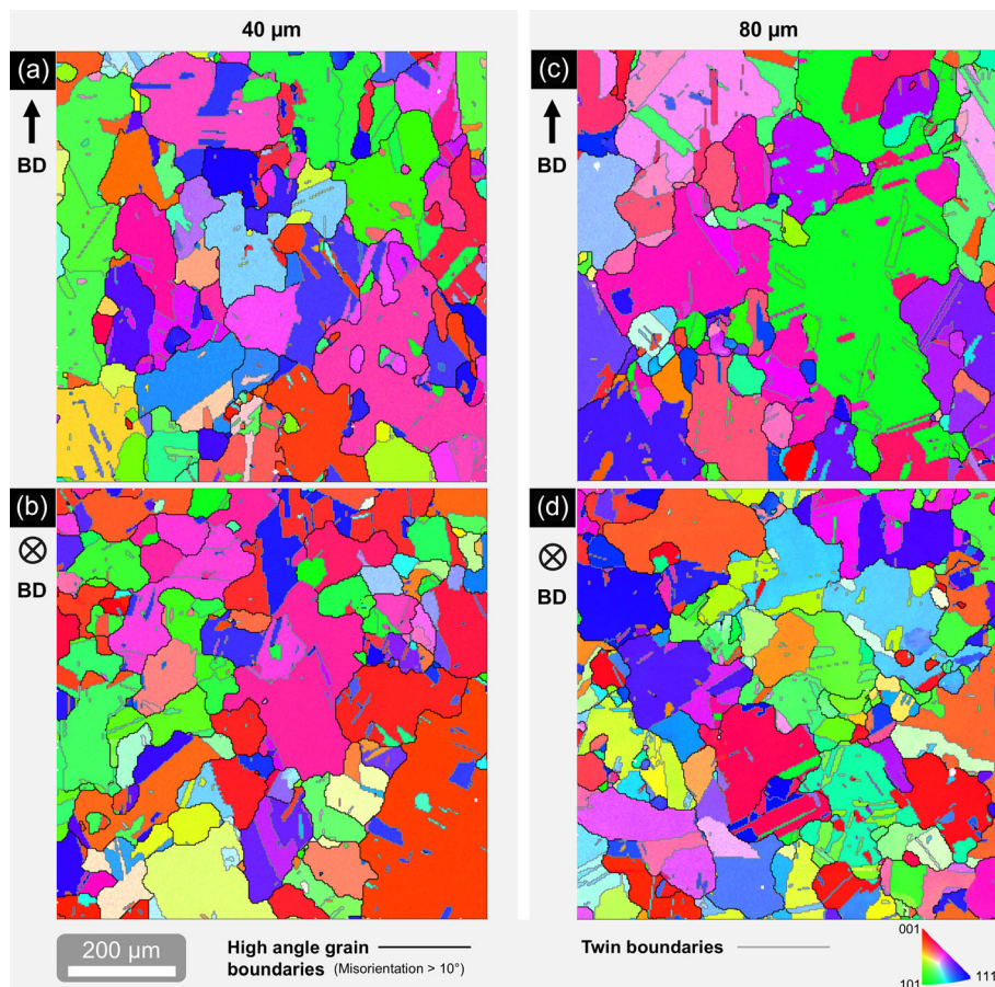
FIGURE 3 | EBSD orientation maps in inverse pole figure (IPF) representation for (a) and (b) 40 μm 282 alloy; and (c) and (d) 80 μm 282 alloy in cross-sections parallel and perpendicular to the BD. IPF coloring is along the BD.
