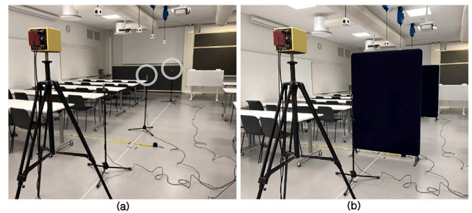
Fig. 6. Photo of room without screening (a) and with screening (b). The receiving microphones at positions 1 & 2 are marked by gray circles in (a), where position 2 is furthest away from the source.
