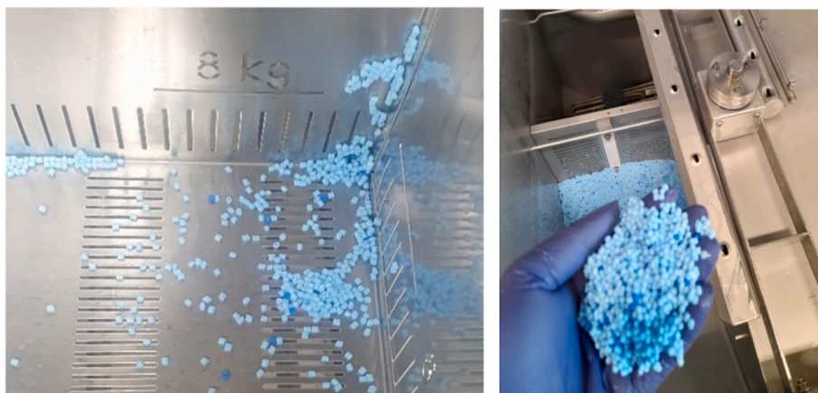
Fig. 4. Plastic pellets for granular coarse dishwashing on ship S2 and S3.
